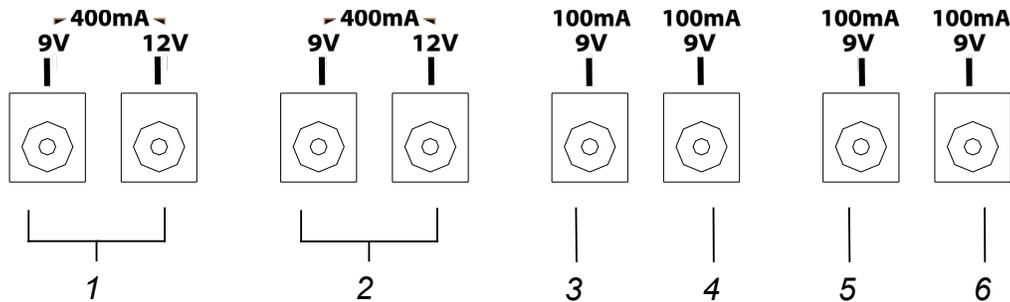
The Hot Stone SMD has 6 isolated outputs. All outputs are standard barrel type connectors wired “center negative”, which means the outside barrel is +V. This is the standard wiring for most guitar effect pedals. However, there are exceptions. Always check the label on the pedal before connecting, and use a polarity reversal cable if needed (see DC Cables section).
